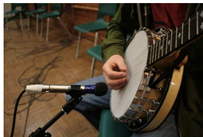
Fig. 5a. Banjo placement: a nice blend of body and strings with room for your picking hand.
