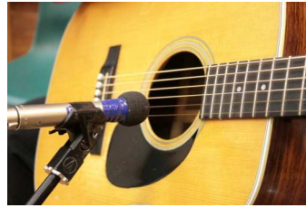
Fig. 3c. Guitar placement: mike pointing at the sound hole is often too boomy and “woofy” due to the air rushing out.
